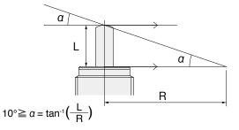
L: Shock absorber's stroke [mm]
