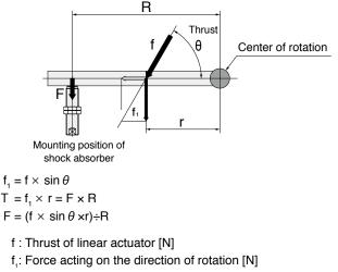
r : Mounting position of actuator's end [m]
