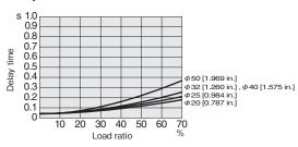
Note: Delay time may vary according to the cylinder stroke.
