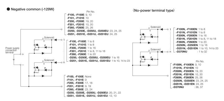
Remark: The internal circuit is of the standard type, For details of the low-current type, see p23.
