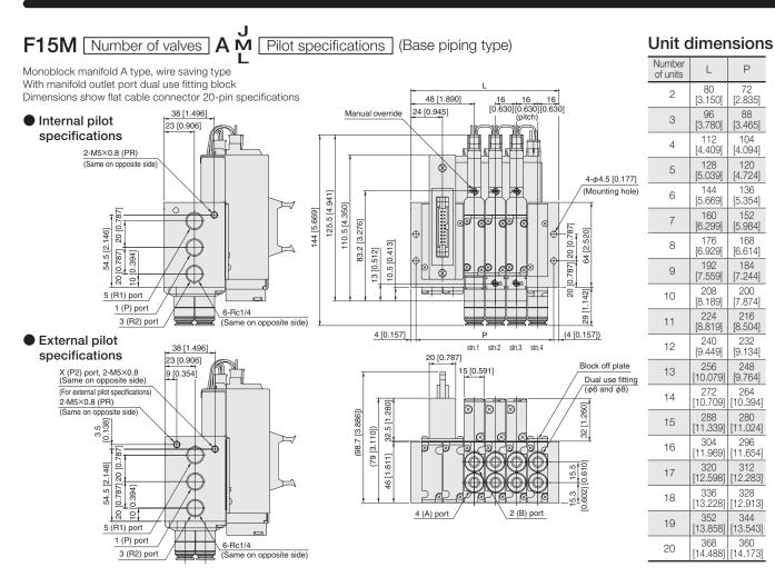
Monoblock manifold A type, wire saving type With manifold outlet port female thread block
