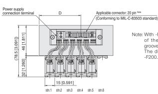
Note: With -F200 and -F201, the positions of the mis-insertion prevention grooves are reversed.
