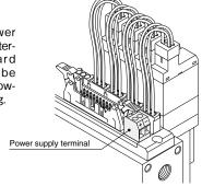
Terminal screw tightening torque: 0.4 N·m [3.5 in·lbf]
