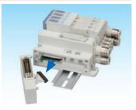
③ Insert the connector to the piping block left.
