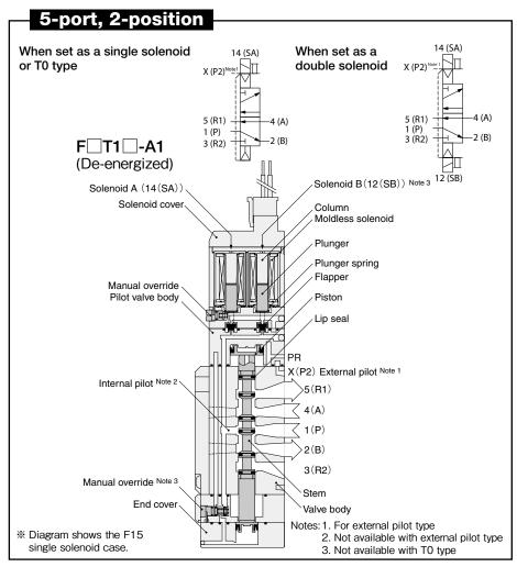
Remark: When using a 5-port valve as a 3-port valve, see p.25.
