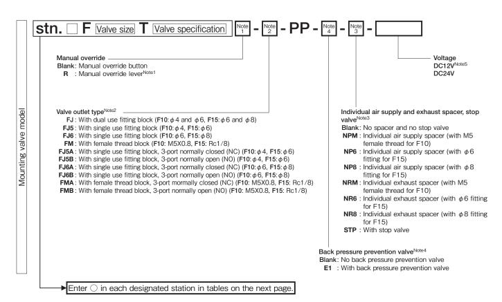
PC Board Manifold F Type (Direct Piping Type)
