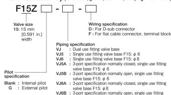
valve base F15: φ8 : Female thread valve base
