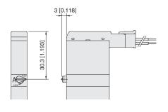
Note: The overall valve length of the T0 type is 8 mm [0.315 in] shorter (end cover side protrusion is 8 mm [0.315 in] less).
