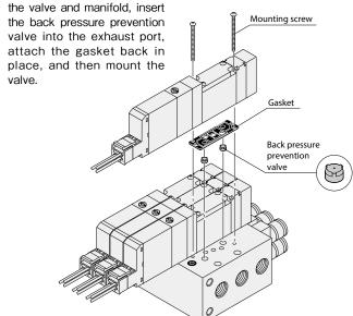
For a split type manifold, insert the back pressure prevention valve into the exhaust port, attach the dedicated gasket and plate provided, and then mount the valve.
