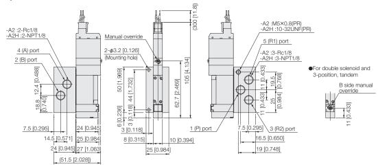
Note: The overall valve length of the T0 type is 8 mm [0.315 in] shorter (end cover side protrusion is 8 mm [0.315 in] less).
