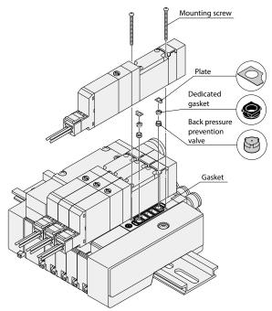
Mounting screw tightening torque: F10 series 17.6 N  $\cdot$  cm [1.6 in·lbf] F15 series 49.0 N  $\cdot$  cm [4.3 in·lbf]
