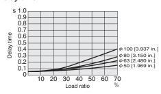
Note: Delay time may vary according to the cylinder stroke.
