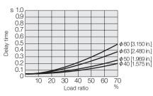
Note: Delay time may vary according to the cylinder stroke.
