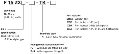
PJ5 : With single use fitting  $\phi 8$ PJ6 : With single use fitting  $\phi 10$ PM : With female thread Rc 1/4 PMH : With female thread NPT 1/4
