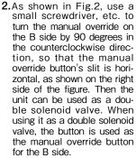
Caution: When using it as a double solenoid valve, do not attach the cover that was removed in
