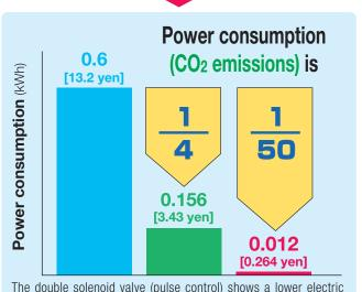
The double solenoid valve (pulse control) shows a lower electric energy result. Note that with higher operation frequency, this difference will narrow somewhat.
