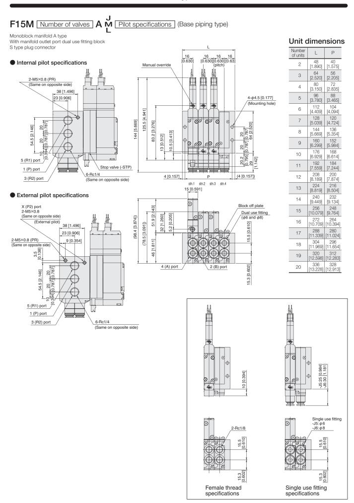
Monoblock manifold A type With manifold outlet port female thread block S type plug connector
