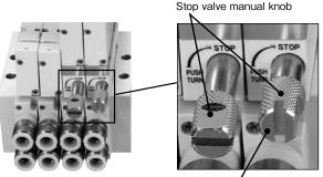
Stop valve manual knob is locked, and air supply shut off.
