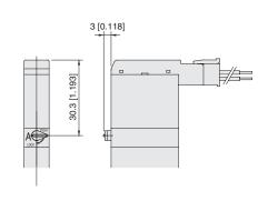
Note: The overall valve length of the T0 type is 10 mm [0.394 in] shorter (end cover side extension is 10 mm [0.394 in] less).
