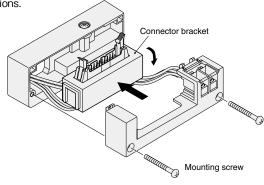
Mounting screw tightening torque: 49 N·cm [4.3 in·lbf]
