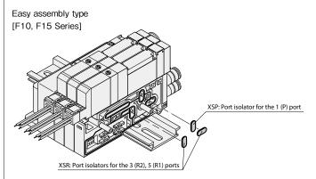
Caution: Installing port isolators requires the disassembly and re-assembly of manifolds. See the disassembly illustration, unit adding procedure, and cautions on p.30-37.
