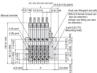
Note: The overall valve length of the T0 type is 8 mm [0.315 in] shorter (end cover side protrusion is 8  $\,$ mm [0.315 in] less).
