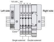
Number of units: 4 units Wiring specification: -F101 Wiring connection specification: -W (double wiring)
