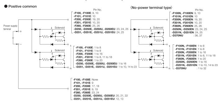
Remark: The internal circuit is of the standard type, For details of the low-current type, see p23.
