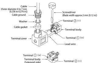
\*For the DC24V solenoid with surge suppression, connect (+) to terminal ①, and (-) to terminal ②.
