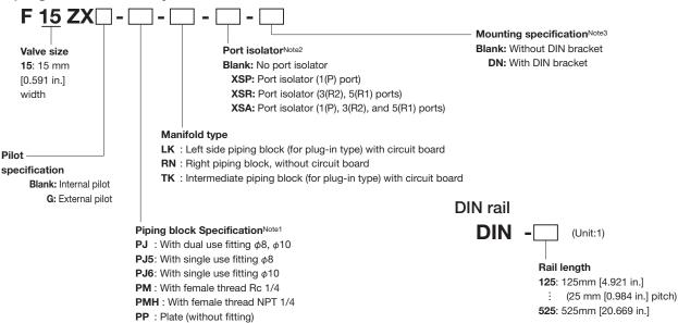
Notes: 1. The fitting of the piping block is included. One set of two connecting rods is also included for a LN and TN type manifold.
