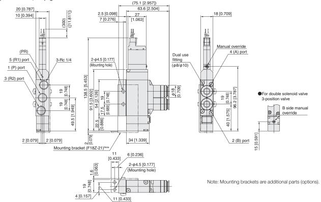
F18T Valve specifications -F4-PS F18T Valve specifications -F4H-PS
