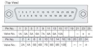
Note: For the no-power terminal type, set pins No.20, 21, and 22 to NC (unused pins).
