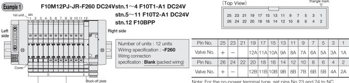
Note: For the no-power terminal type, set pins No.23 and 24 to NC (unused pins).
