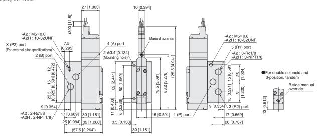
Note: The overall valve length of the T0 type is 10 mm [0.394 in] shorter (end cover side extension is 10 mm [0.394 in] less).
