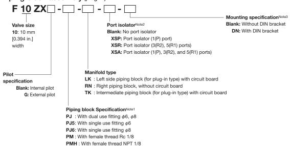
Notes: 1. The fitting of the piping block is included. One set of two connecting rods is also included for a LN and TN type manifold.
