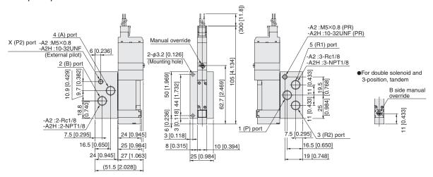
Note: The overall valve length of the T0 type is 8 mm [0.315 in] shorter (end cover side protrusion is 8 mm [0.315 in] less).
