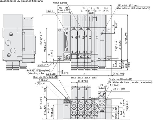
Remark: Add 21 [0.827] to the L and P dimensions right when two of the piping blocks are used.
