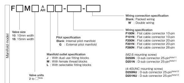
Note: For the maximum number of units, check the table for maximum number of valve units by wiring specification on page 51.
