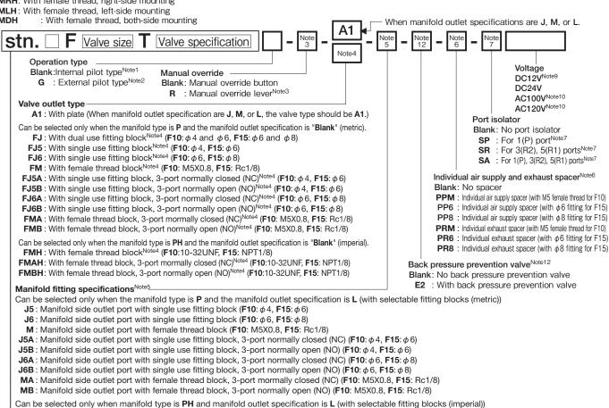
MH: Manifold side outlet port with female thread block (F10:10-32UNF, F15: NPT1/8)
