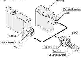
Cautions: 1. When removing the connector, confirm that the lever claw is positively disengaged from the protruded section before pulling out. The housing may be damaged if it is pulled out while engaged with the protruded section.
