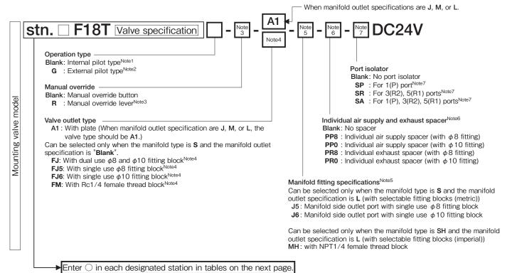
Split Manifold Serial Transmission Type
