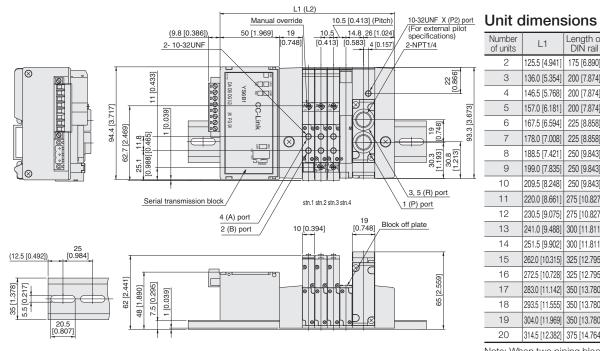
DIN rail mounting hole dimensions
