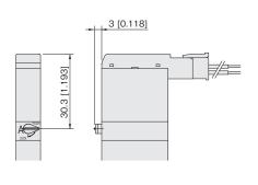
Note: The overall valve length of the T0 type is 12 mm [0.472 in] shorter (end cover side protrusion is 12 mm [0.472 in] less).
