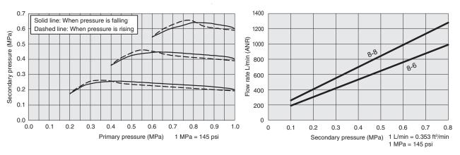
Note 1: Fluctuation of primary pressure 1.0 MPa [145 psi]→Rated pressure (0.2, 0.4, 0.6 MPa [29, 58, 87 psi])→1.0 MPa [145 psi]. 2: Flow rate from secondary side  $\rightarrow$  primary side.
