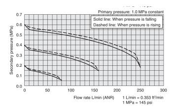
■ Pressure characteristics Note 1 RTUP4-4, RTUP4-4-G RTUP6-4, RTUP6-4-G
