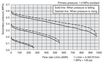
■ Pressure characteristics Note 1 RTLP6-02, RTLP6-02-G RTLP8-02, RTLP8-02-G
