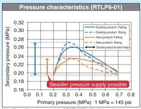
Note: After setting primary pressure: 0.7 MPa [102 psi] and secondary pressure: 0.2 MPa [29 psi], fluctuation of primary pressure: 0.7 MPa [102 psi]→ 0.2 MPa [29 psi]→0.7 MPa [102 psi].
