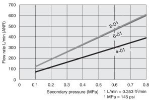
Note 1: Fluctuation of primary pressure 1.0 MPa [145 psi]→Rated pressure (0.2, 0.4, 0.6 MPa [29, 58, 87 psi])→1.0 MPa [145 psi]. 2: Flow rate from secondary side → primary side.
