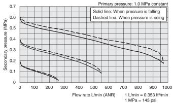
■ Pressure characteristics Note 1 RTUP8-6, RTUP8-6-G RTUP8-8, RTUP8-8-G
