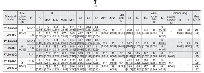
Note: The L1 and L2 dimensions for the tapered threads for pipes are reference dimensions for after tightening.
