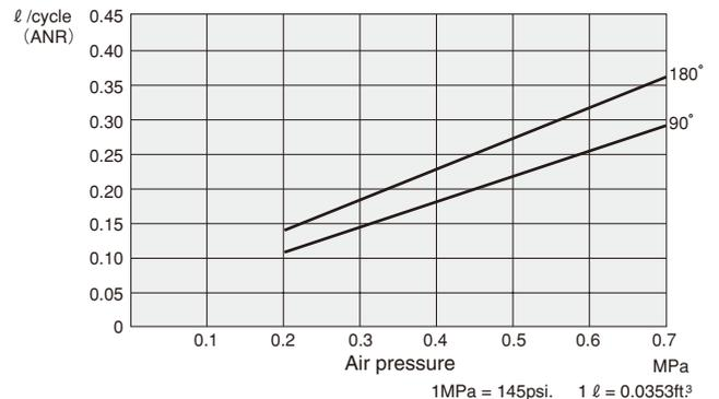
Air consumption per 1 cycle of the rotary actuator can be found by the following equation.
