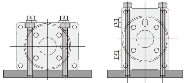
Mounting using the tapped holes on the body
