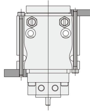
Mounting using the through holes on the body (pattern B)
