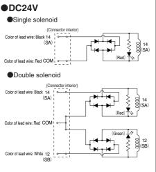
Note:Since there is no polarity, the valve can be used for either +COM or -COM.
