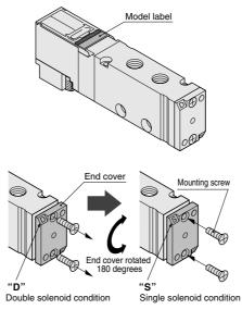
Recommended tightening torque for mounting screws: 88.3N·cm {9.0kgf·cm} [7.8in·lbf]
