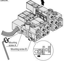
Recommended tightening torque for mounting screws: 411.9N • cm {42.0kgf • cm} [36.5in • lbf]
