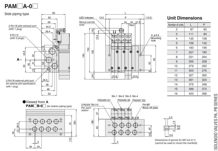
Note: The side piping type and bottom piping type cannot be selected on the same manifold. Select either piping type for the manifold.
