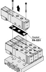
Recommended tightening torque for mounting screws: 176.5N • cm {18.0kgf • cm} [15.6in • lbf]
