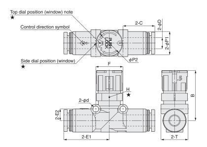
Note: Tube size 4 ( $\phi$ 4 [0.157]) does not have a dial on top.
