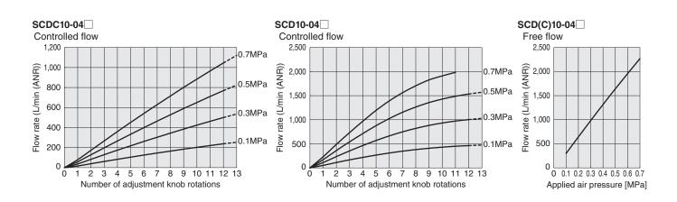
Note: The final speed should be checked occasionally, since it will depend on the individual difference of the product, individual difference of the actuator, and operating conditions such as temperature.
