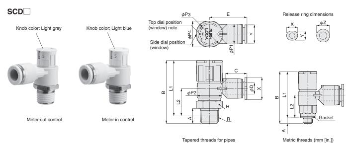
Note: Thread sizes M3 and M5 (metric threads) do not have a dial on top.
