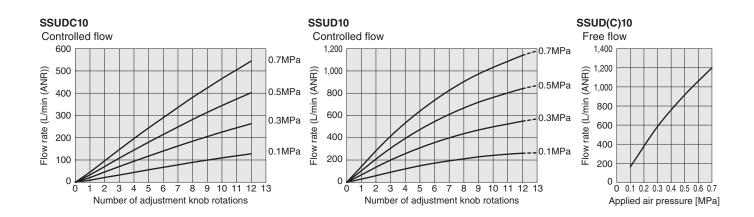
Note: The final speed should be checked occasionally, since it will depend on the individual difference of the product, individual difference of the actuator, and operating conditions such as temperature.
