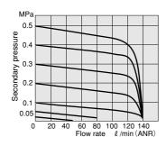
Remark: Graph shows flow rate characteristics when the primary pressure is fixed at 0.7MPa [102psi.].
