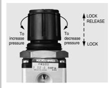
Cautions: 1. The precision regulator is a bleed type, which means that a slight amount of air constantly bleeds out from the bleed hole while the secondary side is under pressure regulation. This is a normal situation.
