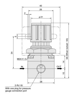
Remark: Mounting holes for installing PR100 on a panel are  $\phi$  24.5.
