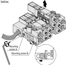
Recommended tightening torque for mounting screws: 411.9N • cm {42.0kgf • cm} [36.5in • lbf]
