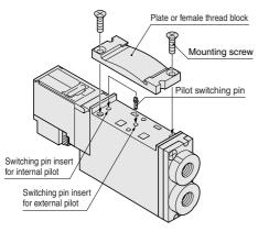
Recommended tightening torque for mounting screws: 137.3N·cm {14.0kgf·cm} [12.2in·lbf]
