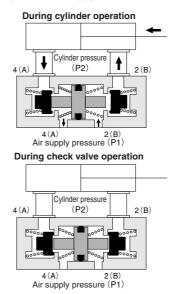
Cautions: 1. Set the cylinder load so that the pressure on the cylinder side 2(B) and 4(A) ports is less than double the supply side pressure and also does not exceed the allowable pressure range.
