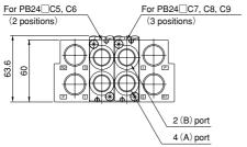
● Dustproof conduit cap: For serial transmission (-FS1)
