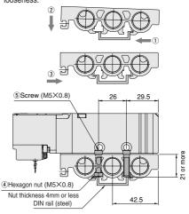
Recommended tightening torque for mounting screws: 284.4N · cm {29.0kgf · cm} [25.2in · lbf]
