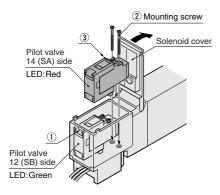
Caution: The maximum height of the cover when open is 48mm [1.89in.] from the top surface. Ensure enough space for maintenance, etc.
