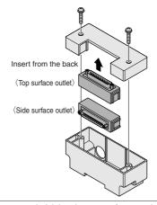
Recommended tightening torque for mounting screws: 58.8N • cm {6.0kgf • cm} [5.2in • lbf]
