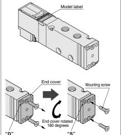
Recommended tightening torque for mounting screws: 88.3N·cm {9.0kgf·cm} [7.8in·lbf]
