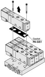
Recommended tightening torque for mounting screws: 176.5N · cm {18.0kgf · cm} [15.6in · lbf]
