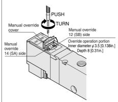
Cautions: 1. The PA/PB series valves are pilot type solenoid valves. As a result, the manual override cannot switch the main valve without air supplied from the 1(P) or X(P2) port.
