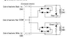
Note:Since there is no polarity, the valve can be used for either +COM or -COM.
