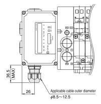
●Individual air supply and exhaust spacer (PB-Z□)
