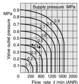
When the supply pressure is 0.5MPa [73psi.] and the flow rate is 740  $\ell$  /min [26.1ft.3/min.] (ANR), the valve outlet
