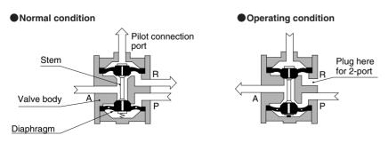
Note: The AA type (internal pilot holding type) is identical, except for the bypass hole (small hole)
