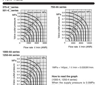
When the supply pressure is 0.5MPa [73psi.] and the flow rate is 12000  $\ell$  /
