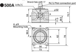
Note: For the normally open type, the exhaust port (R) becomes the inlet port (P), and P becomes R.
