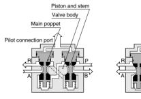
Note: The AA type (internal pilot holding type) is identical, except for the bypass hole (small hole) on the A side stem. For the operating principles and usage, see p.940.
