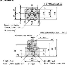
Notes: 1. To change the speed controller installed position to the A port side, just rotate the valve body by 180 degrees. In this case, B becomes NC, while A becomes NO.
