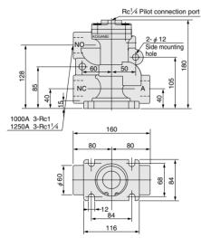
Note: For the normally closed type, the exhaust port (R) is on the NO side. For the normally open type, the exhaust port (R) is on the NC side. (A type only).
