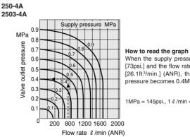
When the supply pressure is 0.5MPa [73psi.] and the flow rate is 740  $\ell$  /min [26.1ft<sup>3</sup>/min.] (ANR), the valve outlet pressure becomes 0.4MPa [58psi.].
