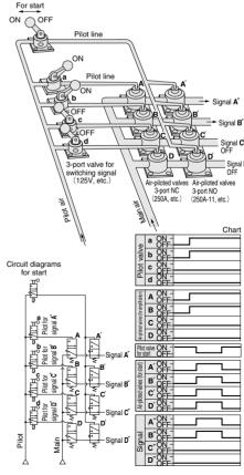
To obtain signals A" and B", turn ON hand operated valves a and b, and open the air-piloted valves A and B. Then, turning off the manual valve for start (which is normally left ON) turns off all of the air-piloted valves, (NO valves) A', B', C', and D', and opens them up, and signals A" and B" appear.
