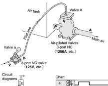
Diaphragm type basic construction (125A type)
