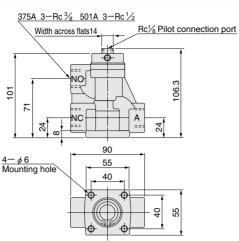
Note: For the normally closed type, the exhaust port (R) is on the NO side. For the normally open type, the exhaust port (R) is on the NC side. (A type only).
