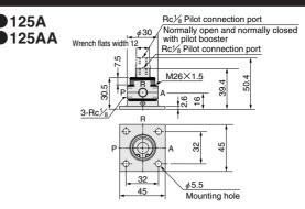
Note: For normally open type, the exhaust port (R) is on the opposite side (A type)
