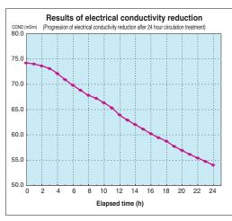
The DB Scale Separator physically removes various kinds of components in raw water, and reduces electrical conductivity (COND: mS/m). For example, in the case of cooling towers, blow down volume, make-up water volume, and sewage amount can be reduced.
