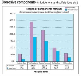
The DB Scale Separator physically removes various kinds of components in raw water by using the special electrolysis method. Especially ionized silica, hardness components, chloride ions, and sulfate ions etc. are simultaneously removed.
