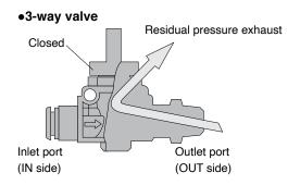
The 3-way valve can exhaust residual pressure (residual pressure remained in installed equipment) left behind in the outlet port side when air has been shut off.
