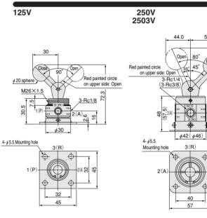
Notes: 1. Although the 125V lever is set on the 1(P) port side in the normal Autodigin the resonance in second the r(r) port side condition, it can be positioned in 360° range.
