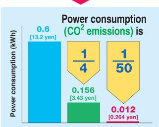
The double solenoid valve (pulse control) shows a lower electric energy result. Note that with higher operation frequency, this difference will narrow somewhat. With use of 0.1W low-current type, the power consumption is reduced to 1/4.
