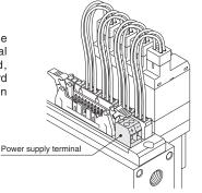
Terminal screw tightening torque: 0.4 N·m [3.5 in lbf] Stripped wire length: 7 mm [0.28 in.] Connecting wire size: 0.13~2.5 mm<sup>2</sup> [0.00020~0.00388 in.<sup>2</sup>] AWG: No.26...14
