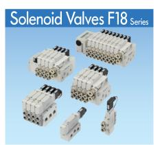
• Valve width: 18 mm [0.709 in.] • Sonic conductance C:  $3.6 \text{ dm}^3/(\text{s}\cdot\text{bar})$  (Cv: 1) • Applicable cylinder bore sizes:  $\phi 50 [1.969 \text{ in.}] \sim \phi 100 [3.937 \text{ in.}]$
