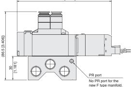
• Optional back pressure prevention valve for both the A type and F type manifolds now available.
