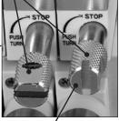
Stop valve manual knob is locked, and air supply shut off.
