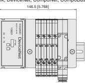
Stand alone type (flat cable connection) (Compatible with OMRON B7A Link Terminal)
