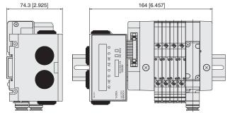
\*While dimensions show F10 Series, the F15 Series is similar. ■ Reference photo: Valve base assembly (Photo shows F10 Series.)
