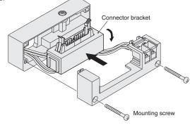
Mounting screw tightening torque: 49 N·cm [4.3 in·lbf]
