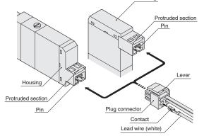
Cautions: 1. When removing the connector, confirm that the lever claw is positively disengaged from the protruded section before pulling out. The housing may be damaged if it is pulled out while engaged with the protruded section.
