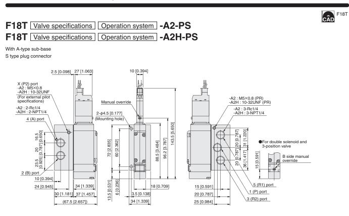
Note: The overall valve length of the T0 type is 12 mm [0.472 in] shorter (end cover side protrusion is 12 mm [0.472 in] less).
