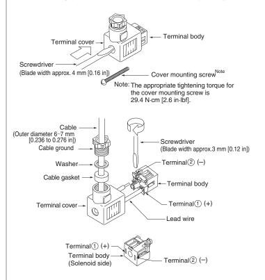
\*\*For the DC24V solenoid with surge suppression, connect (+) to terminal ①, and (-) to terminal ②.
