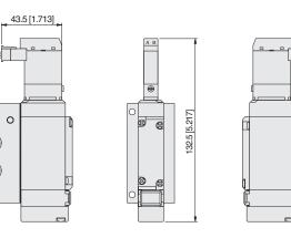
Note: The overall valve length of the T0 type is 12 mm [0.472 in] shorter (end cover side protrusion is 12 mm [0.472 in] less).
