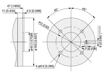
S6 (VYP10S6L) (for mounting ISO standard flange 6, pitch diameter 80 [3.150])
