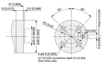
S4 (VYP03S4L) (for mounting ISO standard flange 4, pitch diameter 50 [1.969])
