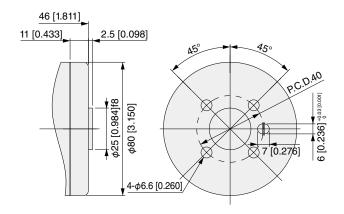
S5 (VYP05S5L) (for mounting ISO standard flange 5, pitch diameter 63 [2.480])
