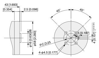
S3 (VYP03S3L) (for mounting ISO standard flange 3, pitch diameter 40 [1.575])
