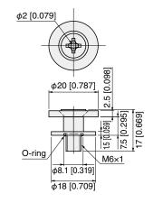
Mounting screws for 5 (M-KPTC5) Mounting screws for 7 (M-KPTC7)
