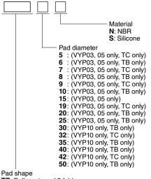
**TB**: Bellows type 1.5 folds **TC**: Bellows type 2.5 folds
