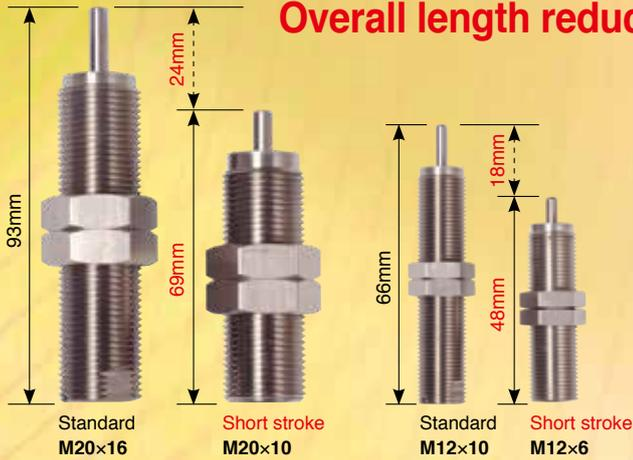
Up to 26% reduction in overall length compared to the same standard threaded body type (for M20). Excellent for absorbing shocks in tight locations as a stopper between 2 cylinder stroke ends because overall short length. Fine position adjustments are easy with more models available with hex sockets.
